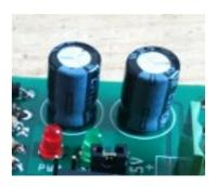
electrolytic capacitors are polarized.
